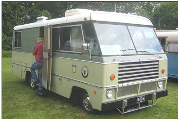
Nancy & Clayton Snyder - Penalosa, KS 1972 Superior 22 ft. Class A Motorhome. The Superior was built from 1970 to about 1978. Construction is all welded galvanized steel. Built on a Dodge M300 chassis, powered by a 413 Dodge truck engine. This unit is original with a few modifications.
