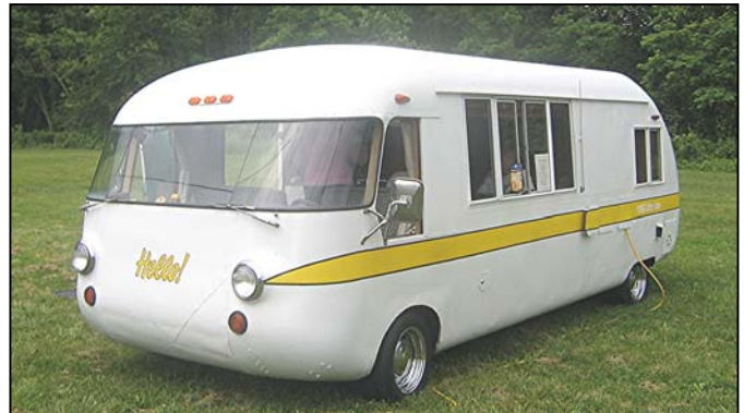
Paul Pieche - Berkley, MI 1968 UltraVan, made in Hutchison, KS, weighs 4,300 pounds. It's made of aluminum with fiberglass corners and Formica paneling. The van is powered by a rear engine 110hp Corvair engine and will cruise at 65 MPH.
