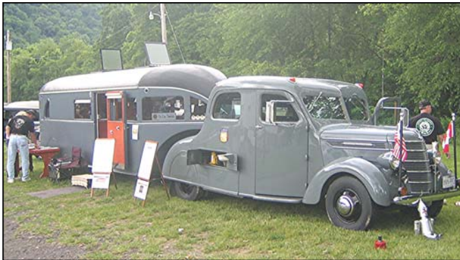
Lana & Ken Hindley - Union, Ontario Canada The Hindley's 1938 International truck is a custom bodied unit with camping features to compliment the 1936 Curtiss Aerocar, a fifth wheel model with no actual chassis and constructed with a fabric covering similar to early airplanes.
