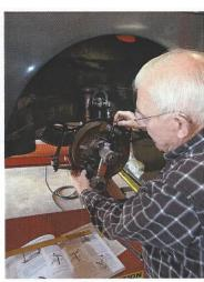
In the picture on the left, the brake tool is applied to the spindle with settings obtained from the brake drum. In the picture on the right, Willis rotates the brake tool to see how well the lining will contact the drum. Major and minor adjustments are made to each shoe for minimal wear and maximum stopping power. The brake adjusting tool came with a brake lathe manufactured by Aamco.
