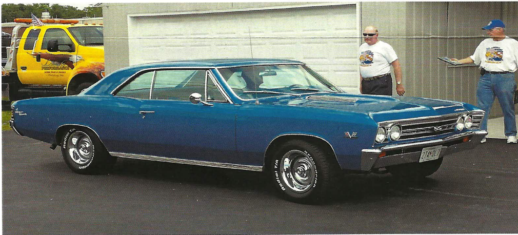
Dave Feinberg is behind the wheel in this recent photograph, shortly after restoration was completed. Dave restored his 1967 Chevrolet Chevelle Super Sport two-door hardtop with a 454 c.i., crate motor with aluminum heads and 'Tremec' five speed transmission with overdrive. Differential is a Moser twelve-bolt with 3.42 gears. The Chevelle also has aftermarket 'vintage' air-conditioning.
