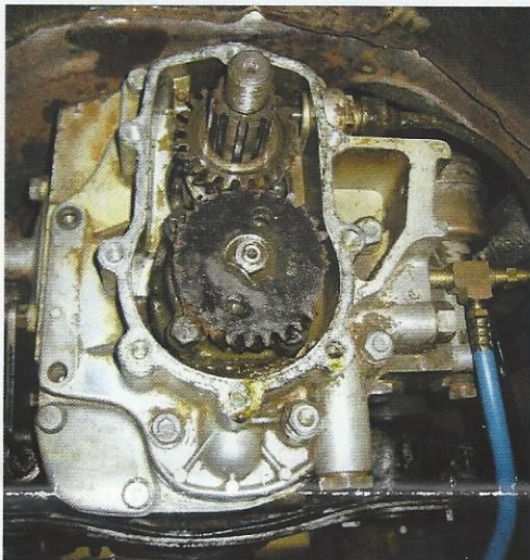
In the picture above, the lower 'fibrous' gear is badly 'chewed' up and is causing 'zero' hydraulic pressure to make shifts properly. The blue hose is attached to a gauge to test pressure during shifts. Murray Cole 'jabbed up' a unique connector to fit the port on the transmission for the hose.
