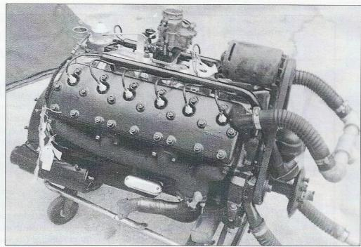
This is the original twelve cylinder flathead motor that came in the Lincoln Continental that Larry purchased. Fortunatly, it was saved intact after it was replaced with an overhead valve V8. Larry rebuilt the flathead and reinstalled it in the '47. The engine stand the motor is resting on began life as a 'shopping cart.'
