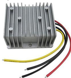
Because my 1950 Ford has a positive ground, I attached a wire to the negative pole on the accessory switch through a fuse to the negative input wire on the converter. The positive input wire on the converter is grounded. These connections would be reversed if the car had a negative ground system. I used
